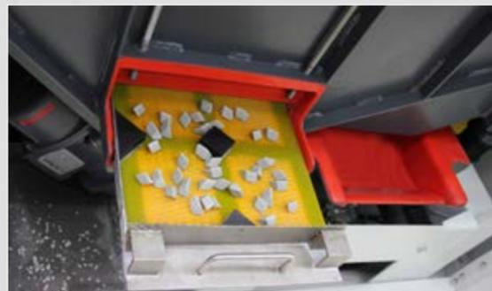
Undersize media classification with flexible, self cleaning "flapper" screen.
