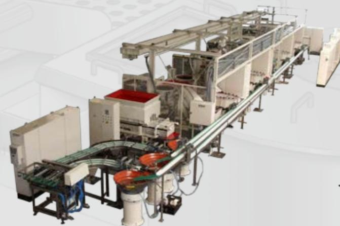
Linked system (4 tandem units) with special 6 track work piece channeling device for transport to the subsequent washing machine
