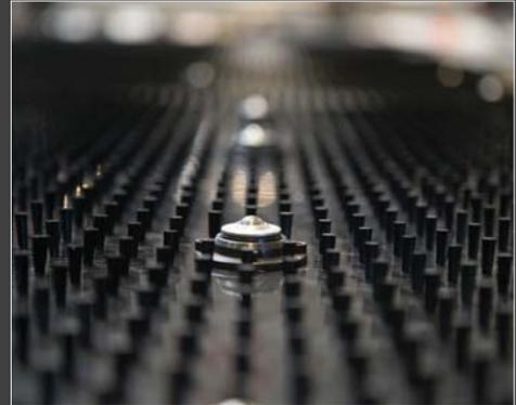
■ Workpieces are manufactured without damaging and smoothly thanks to special brush system
