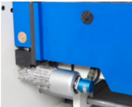
Motorized folding beam adjustment as 80 mm.
