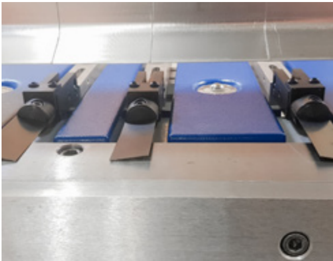
Solid lower beam tool with feather grooves.
