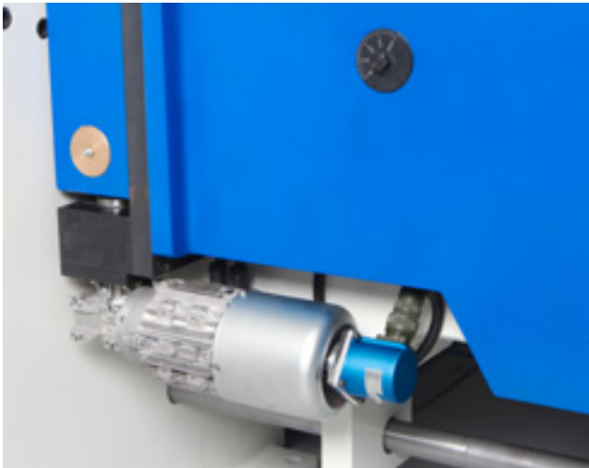
Motorized folding beam adjustment as 80 mm.
