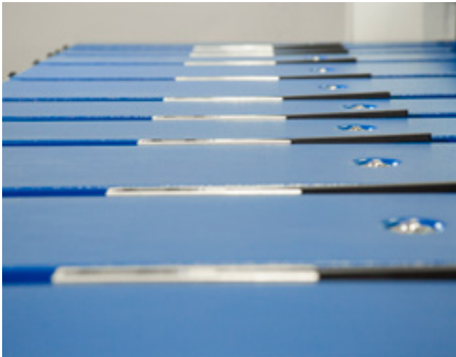
1000 / 1500 mm motorized back gauge system and sheet support table with ball casters.
