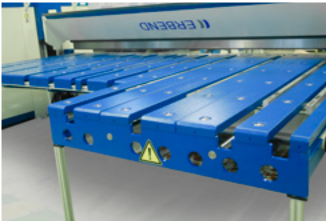
L shape back gauge system (metal or with brushes).
