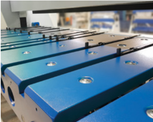
1500 / 2000 / 3000 mm motorized back gauge system and sheet support table with ball casters.
