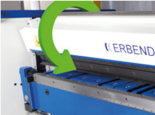
250 mm stroke capacity on 180° rotating combi clamping beam with 2 tooling stations as 120 mm high segmented goat foot tools on station 1 and 20° single piece sharp nose tool on station 2.
