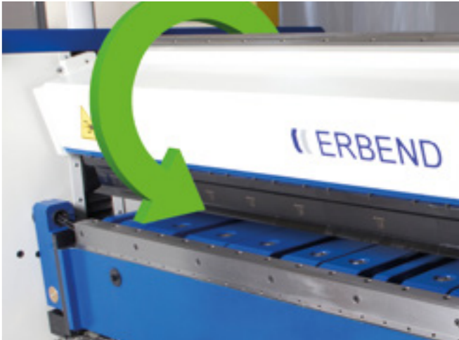
180° rotating clamping beam with 350 mm stroke capacity and 2 tooling stations as 170 mm high segmented goat foot tools on station 1 and 20° single piece sharp nose tool on station 2.
