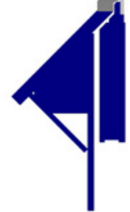
Beam geometry with goat foot
