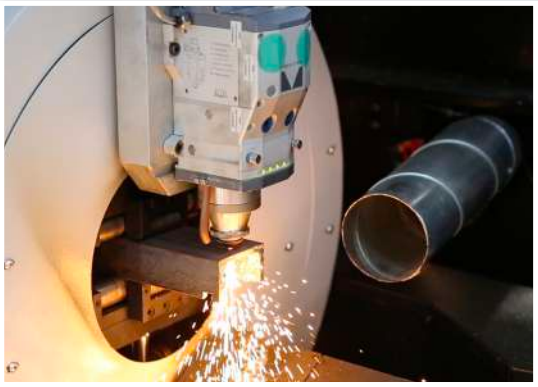
Pipe and profile cutting option allows to cut the pipe, square, rectangular, "U" and "L" shaped profiles.
