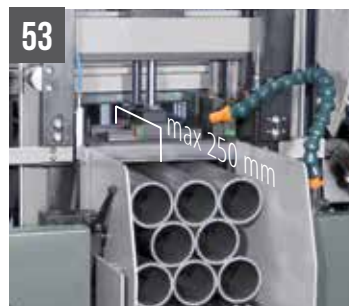
53 SHARK 230-1 NC HS 5.0 Hydraulic vertical vices for bundle cutting (max 230x230 mm)
