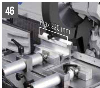
46 COBRA 352 NC 5.0 Special vice to reduce restpiece
