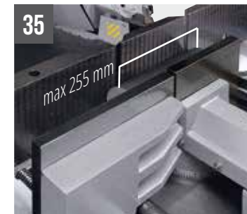
SHARK 332-1 NC 5.0 Special vice to reduce restpiece
