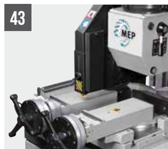
TIGER 352MA/SXevo/NC 5.0 TIGER 372 SXevo Supplementary pneumatic vice
