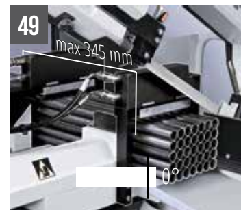
49 SHARK 281 NC 5.0 Hydraulic vertical vices for bundle cutting (max 170x130 mm)
