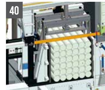
40 SHARK 660 CNC HS 4.0 Hydraulic vertical vices for bundle cutting (660 x 660 mm)
