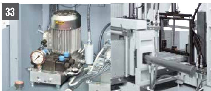
SHARK 350 CNC HS 4.0 - Hydraulic vertical vices for bundle cutting (max 350x350mm)
