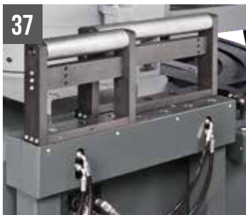
37 SHARK 652 SXI H 5.0 Hydraulic pop-up roller right
