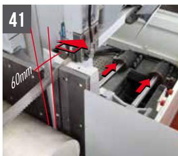
41 SHARK 660 CNC HS 4.0 Retractable fixed vice jaw
