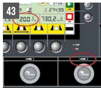
43 SHARK 420 CNC HS 4.0 / SHARK 350 CNC HS 4.0 / SHARK 350 NC HS 5.0 Kit cutting speed 15÷200 m/min
