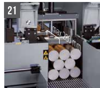
SHARK 420 CNC HS 4.0 - Hydraulic vertical vices for bundle cutting (max 400x400mm)
