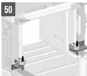
50 Shark 350 CNC hs 4.0 / SHARK 350 NC hs 5.0 Bar sensor to optimize restpiece (3 special cutting cycle)
