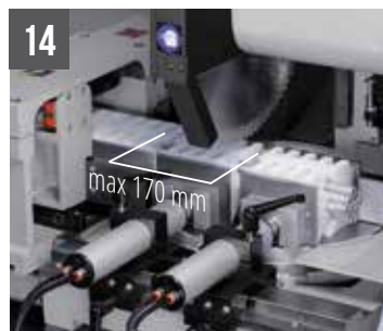
TIGER 402 CNC HR 4.0 - Set of comb jaws when equipped w/restpiece reduction min. (max 75x75mm)
