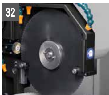
TIGER 372 CNC LR 4.0 (Ø max 105 mm) set of carbide guides
