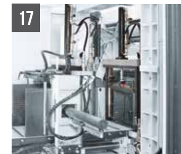
SHARK 350 NC HS 5.0 Hydraulic vertical vices for bundle cutting (max 350x350mm)
